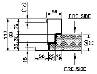
2 hours 3 Criteria Fire Rated Door, fabricated for two hours and three criteria performance in Stability, Integrity and Insulation as per BS 476 Part 22 and IS 3614 Part II, in both directions .
