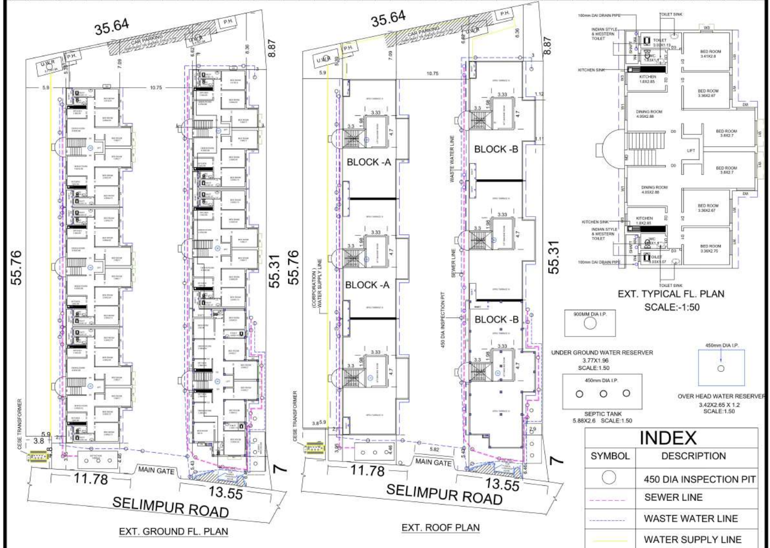
BLOCK WISE SINGLE LINE DIAGRAM OF WATER SUPPLY, SEWER & WASTE WATER LINE
